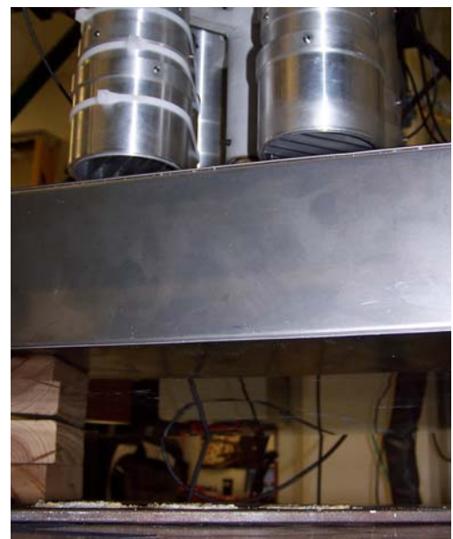
Figure 8 – Steel plate with boric acid deposits positioned 7.62 cm beneath 7.62 cm of TRANSCO insulation
