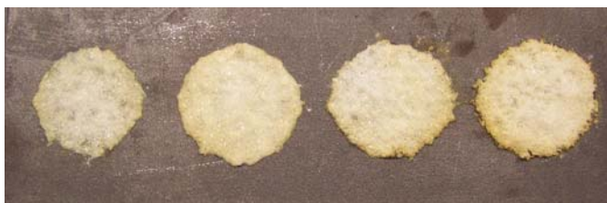
Figure 7 – From left to right, 51, 101, 153, and 204 mg/cm 2 of boric acid in 5 cm diameter circles
