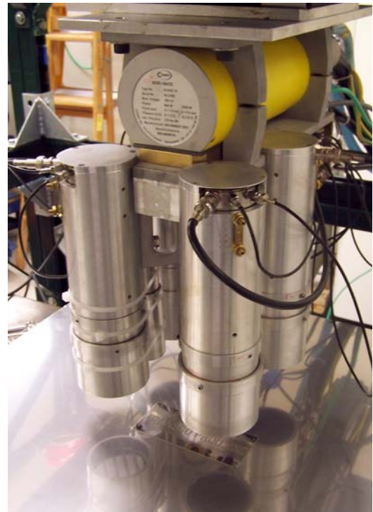
Figure 4 – Current RSD scanning system with TRANSCO mirror insulation
