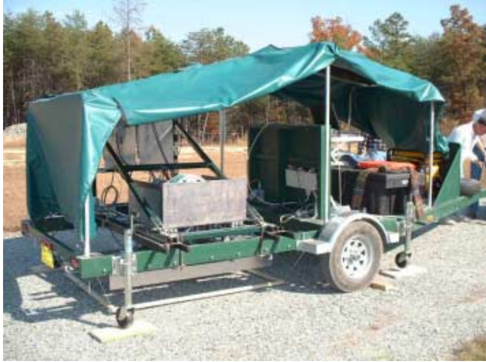
Figure 6. The XMIS in position for image acquisition on mine lane.
